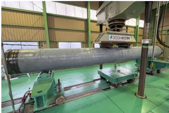
200N pile bending test scene
