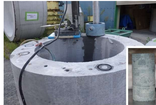
200N pile core sampling
