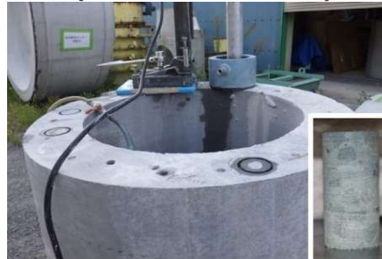
Pile with strength of 200 N/mm 2
