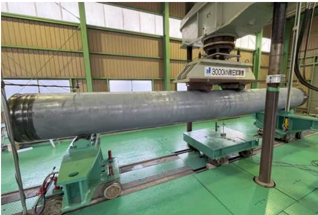
200N pile bending test scene
