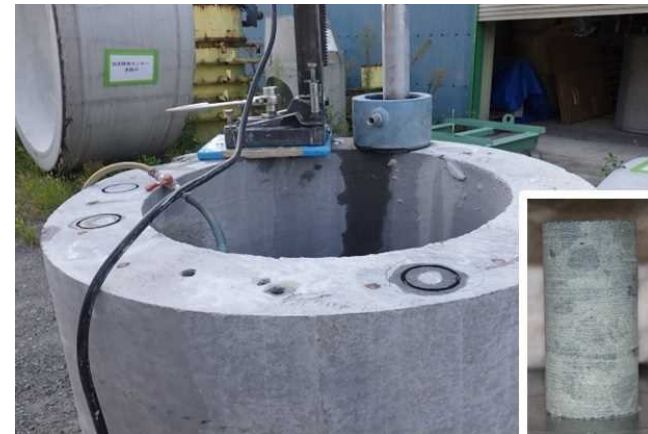
200N pile core sampling
