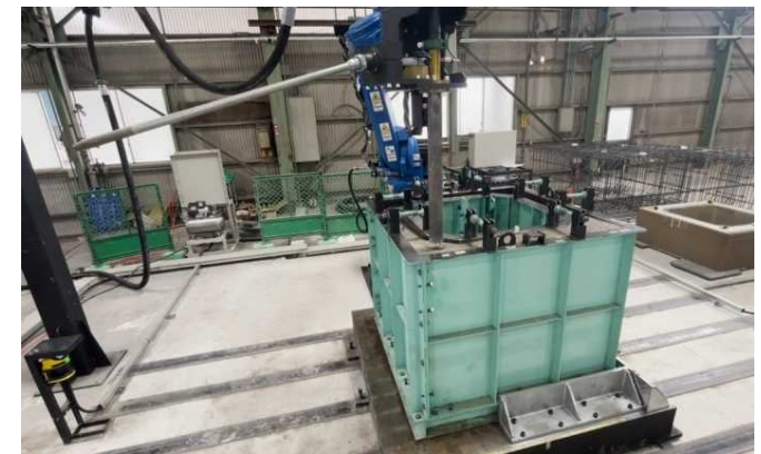
Concrete placement into 3D-printed formwork
