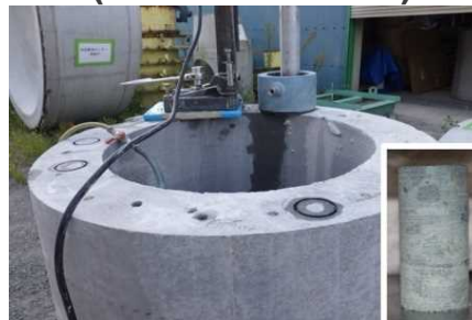
Pile with strength of 200 N/mm 2
