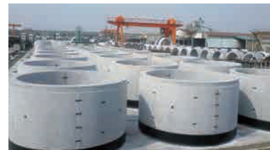
Assembly-Type Super-Large-Diameter Jacking Pipe
